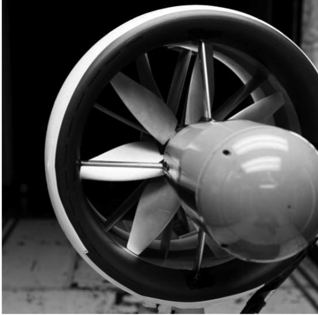
Fig. 16 Leading-edge flow control configuration in the wind tunnel.
