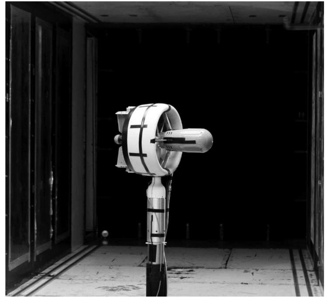
Fig. 14 Vehicle model installed in the Virginia Tech 6 × 6 ft wind tunnel.
