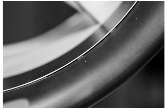
Fig. 15 Coandă trailing-edge flow control slot geometry.
